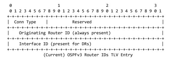
An enhancement below is to allow one entry to represent a number of router IDs or a number of DR IDs. This can be achieved by using two bytes of the Reserved field to indicate the number M of router IDs or a number of DR IDs contained in the entry. The value of the two bytes can be the number of IDs (i.e., M) or the number of octets used (i.e., 4\*M for M router IDs or 8\*M for M DR IDs). The former is preferred.
