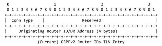
To represent N router IDs or DR addresses, we need N entries, which occupies 8\*N bytes in the OSPFv2 Area Router IDs TLVs. Each entry represents just only one router ID or DR address.
