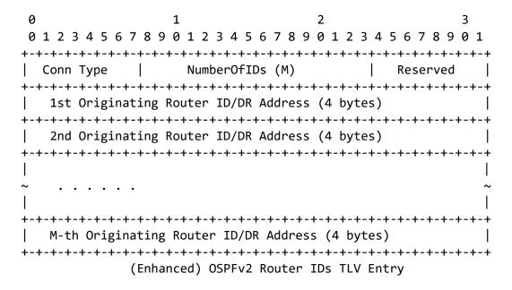
To represent N router IDs or N DR addresses using the enhanced entry, we need just one or a few entries. Using X entries occupies 4\*(N + X) bytes in the OSPFv2 Area Router IDs TLVs.
