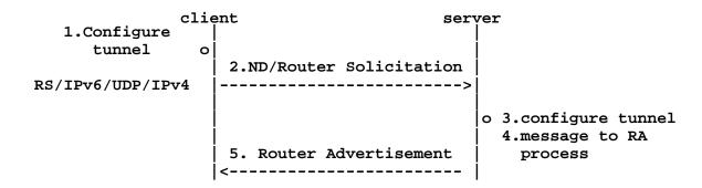
If SEND is used for authentication, Router Solicitation additionally includes the CGA, RSA Signature, Nonce, and Timestamp options. The server has the user's public key in file, and checks the CGA address against that. The fact that the client has been able to sign the ND message with the private key is sufficient for the server to ascertain user's identity.
